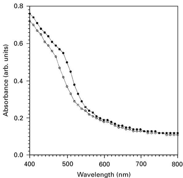
Figure 1 Optical absorption spectra of (○) as-deposited and (●) annealed (at 673 K for 3 h) CdS thin film.
