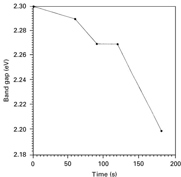
Figure 3 Variation of band gap,  $E_g$ , with annealing time.
