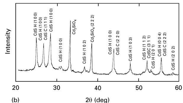
Figure 5 XRD ( $\text{CuK}_\alpha$  radiation) patterns of (a) as-deposited and (b) annealed (at 673 K for 3 h) CdS thin film.
