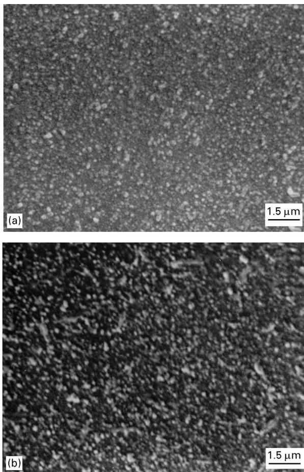
Figure 4 Scanning electron micrographs of (a) as-deposited and (b) annealed (at 673 K for 3 h) CdS thin film.
