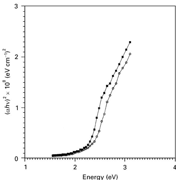
Figure 2 Variation of  $(\alpha hv)^2$  with energy of (○) as-deposited and (●) annealed (at 673 K for 3 h) CdS thin film.
